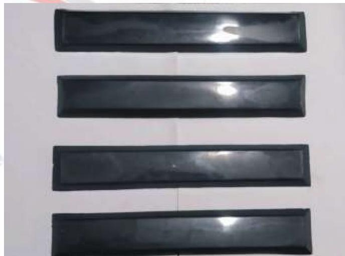
position 6. Lube Bar starts melting at 50 to 60°C and the film smeared on the mating surface, ensure proper lubrication for a longer period.
